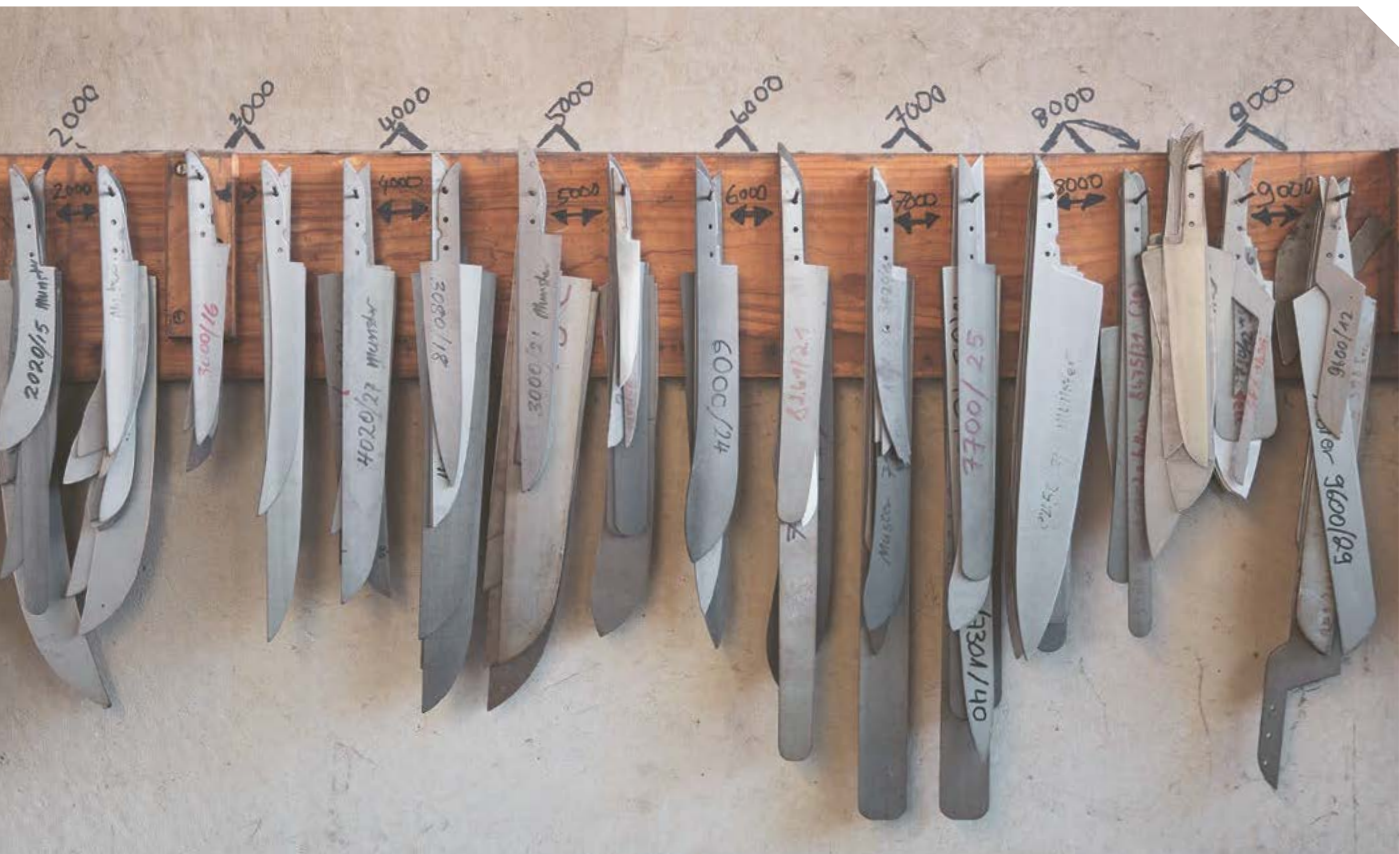
Top High-quality blade blanks from chromoly steel in more than 2,000 designs.
